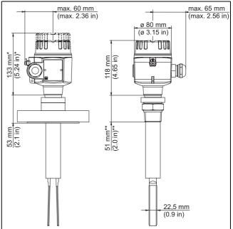
Aluminium housing (T13) with separate connection compartment
