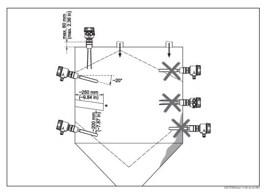
Horizontal installation / Vertical installation
